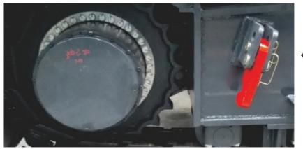
High and low speed travel mode can be switched, and it can travel at low speed with load, safety and reliable.
