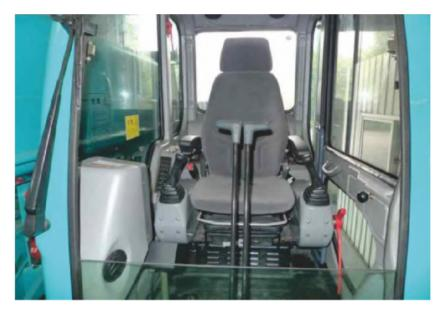
◆ The cab' independent patent pivothung window design, make it has an wide field view, the multi camera video surveillance system has covered all the visual blind area. The cab has air conditioning, capable of being equipped with fuel warm A/C as optional to adapt to the cold region.
