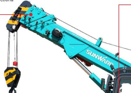
The tail is short and has a small steering radius, particularly suitable for narrow working areas.
