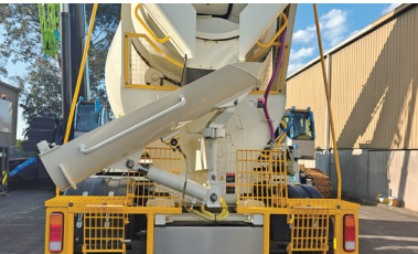
8.Hydraulic Chute Ram with Built-in Safety Valve (control by remote) .
