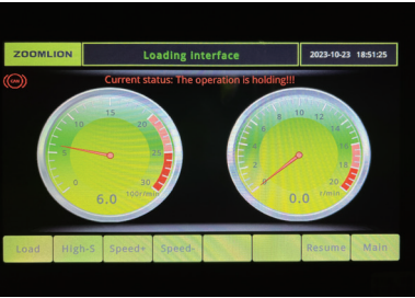
1.MIC (mixer truck Intelligent constant speed control system): Mic system can save more than 6.6% fuel.
