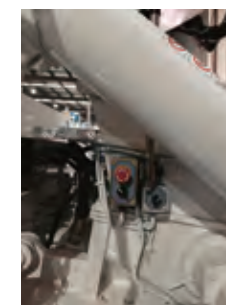
Emergency Button & Water Pump Button on Both Sides of Hopper
