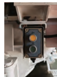
Electric Whistle & Vibrating Motor Buttons on Both Sides of Hopper
