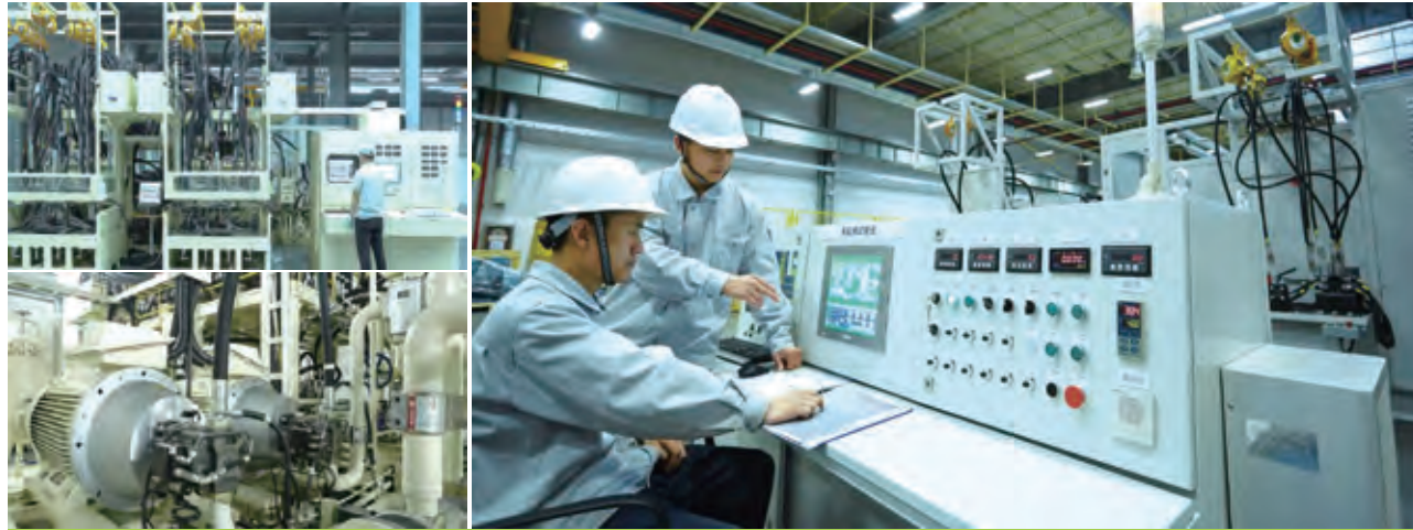
Integrated test bench for hydraulic pumps, hydraulic cylinders, and hydraulic valves
